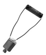
Hold one end of the first wire to the positive (+) end of the AA battery while you hold the other end of that wire to one of the copper contacts on the motor.
